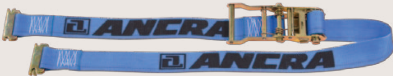
Series E Low Profile Buckle Strap w/ Spring E Fitting Strong 6,000 lbs. polyester webbing. WLL: 1,333 lbs./605 kg. Fixed End: 48-in.
